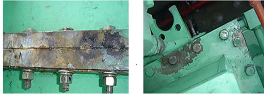
Figure 1. Aftereffect of flange bolt overheating
