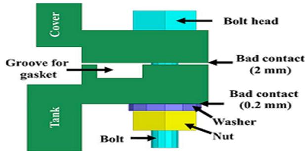
Figure 2. Loose bolt condition
