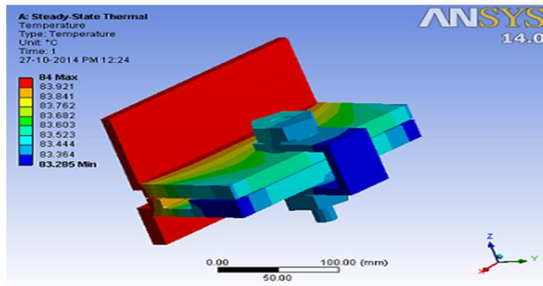
Figure 6. Steady state thermal analysis of flange bolt region without copper link
