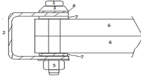
Figure 4. Geometry of the proposed solution. 1. stainless steel bolt IS 1367. 2.copper link. 3. belleville washers, nonmagnetic material AISI-304. 4. flat washers, non-magnetic material IS 2016. 5. stainless steel nut, nonmagnetic material IS 1367. 6. flange for connection of tank and cover IS 2062:2006. 7. toothed washer, nonmagnetic material.
