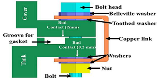
Figure 3. Loose bolt with copper-link
