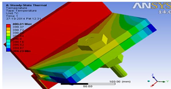
Figure 5. Result showing Steady state thermal analysis of transformer tank's flange bolt region without copper link
